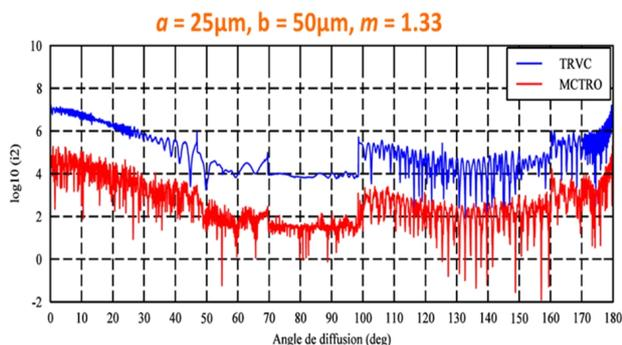
**Figure 3** Comparisons of the scattering patterns of a spheroidal droplet of transversal radius  $b=25 \mu\text{m}$ , symmetric radius  $a=50 \mu\text{m}$  and of refractive index  $m=1.33$  illuminated by a polarized plane wave of wavelength  $\lambda = 0.6328 \mu\text{m}$  calculated by VCRM and MCRTW. The result of MCRTW is shifted by  $10^2$  for clarity.
