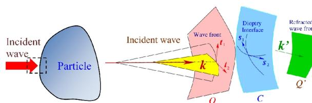
Figure 1 Definition of the curvatures of wave fronts and dioptric surface.
